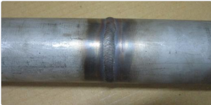
Stainless steel weld before
